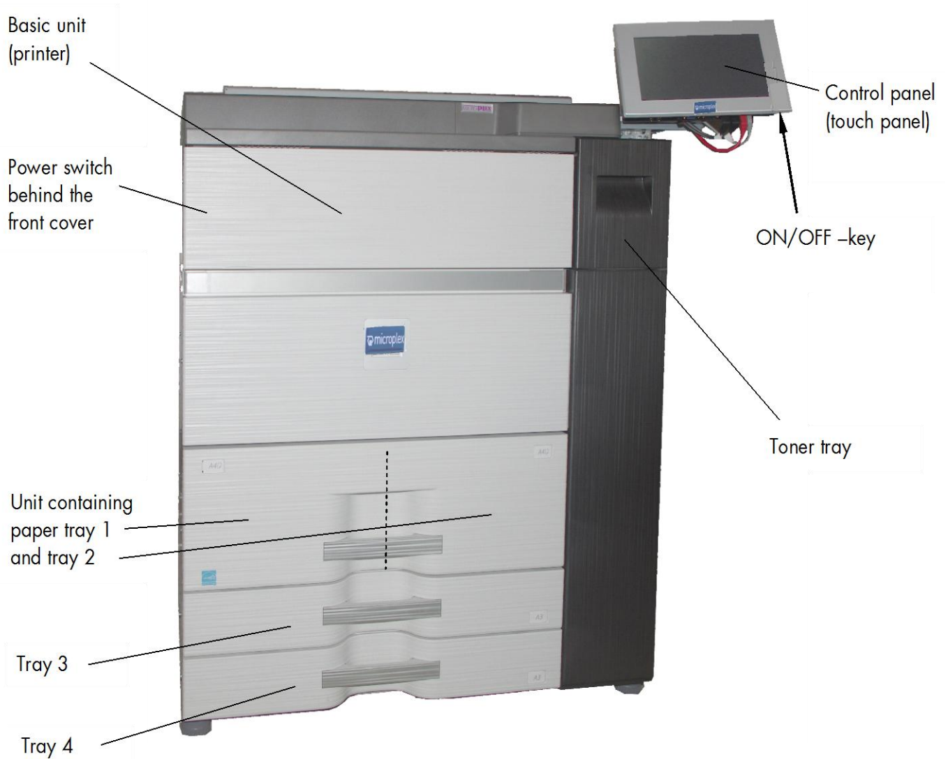
Fig. 2.3.a Print System (for example SOLID 90 A3-2; here without options)
