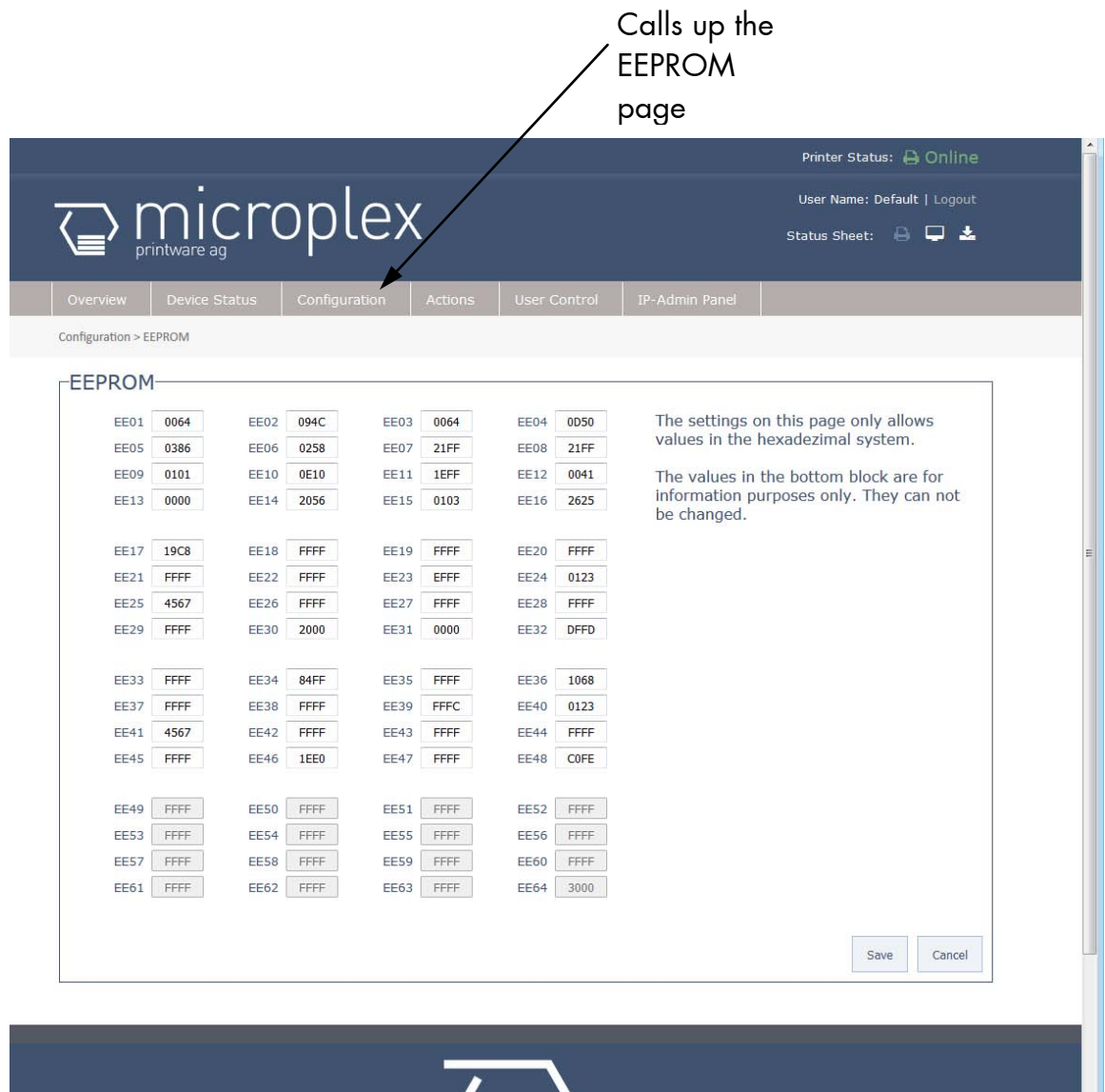
Fig. 6.3.6.a SOLID 90 A3-2/105A3-2/120 A3-2: EEPROM page of the MICROPLEX WebPanel
