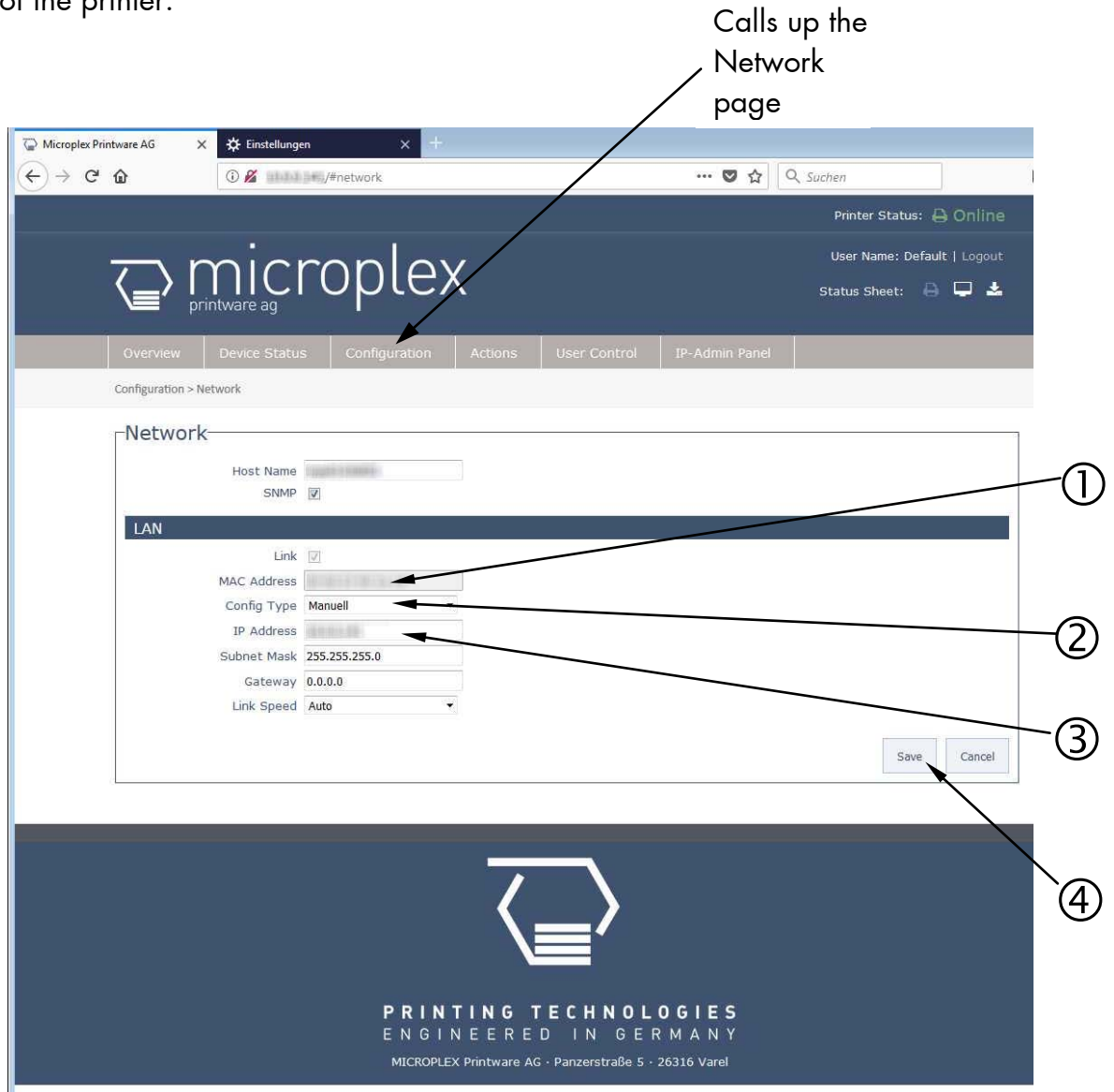
Fig. 6.3.4.a SOLID 90 A3-2/105A3-2/120 A3-2: Network page of the MICROPLEX WebPanel
