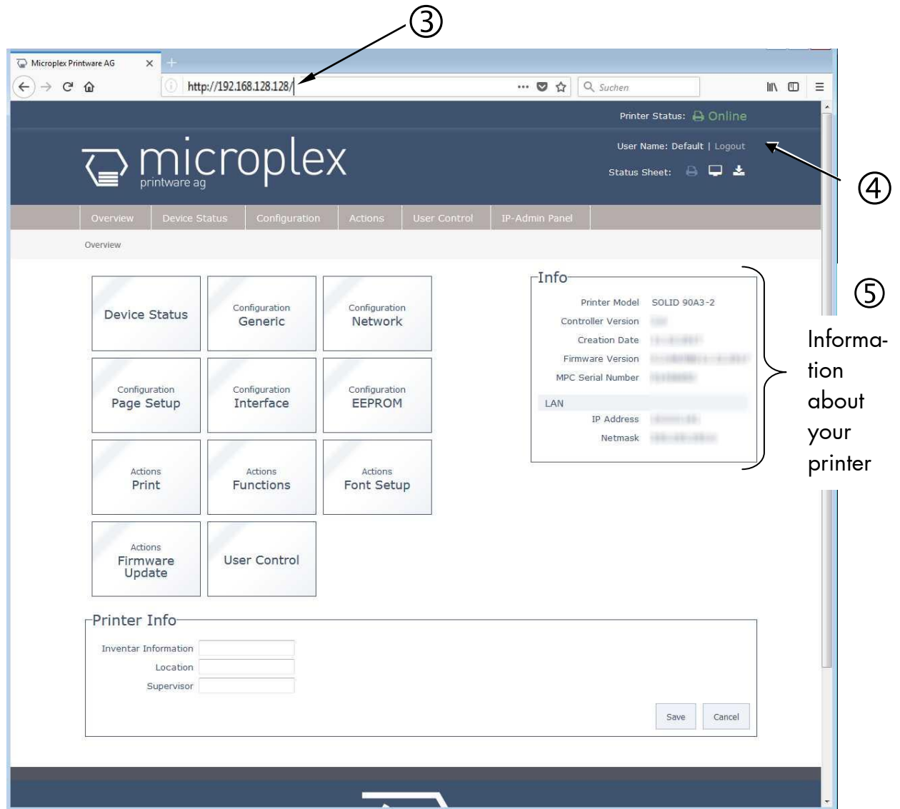
Fig.6.2.a SOLID 90 A3-2/105A3-2/120 A3-2: Overview page of the MICROPLEX WebPanel
