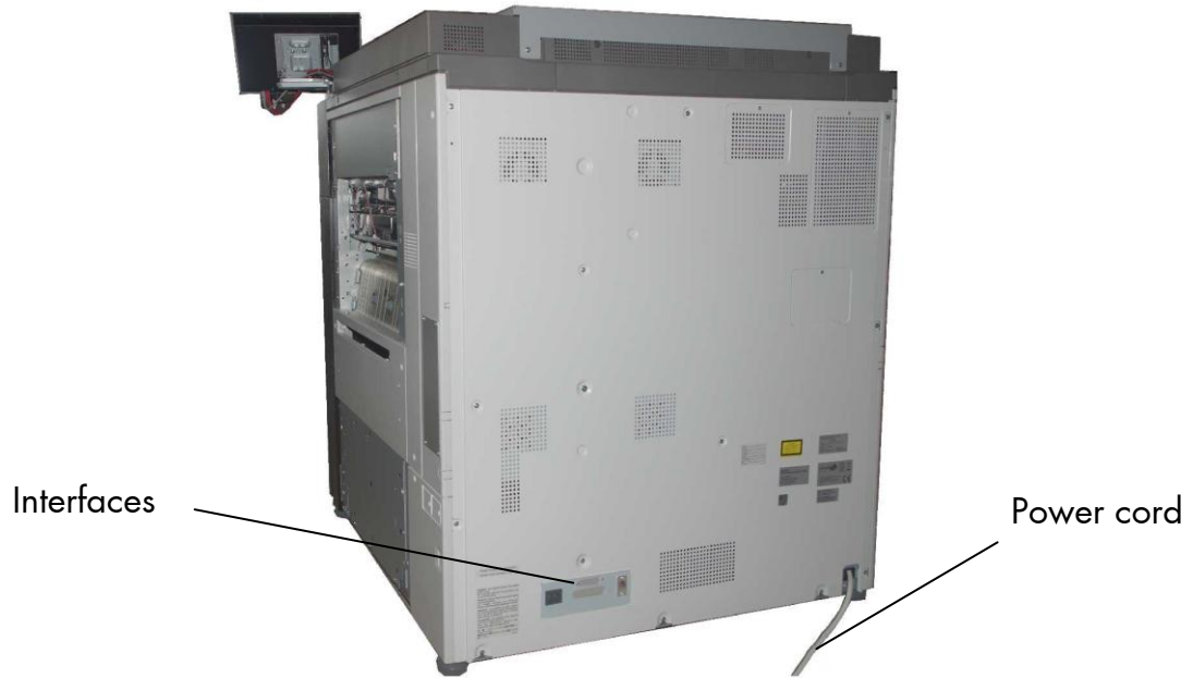
Fig. 4.1.a Rear view of the SOLID 90 A3-2, 105 A3-2 and 120 A3-2 print system
